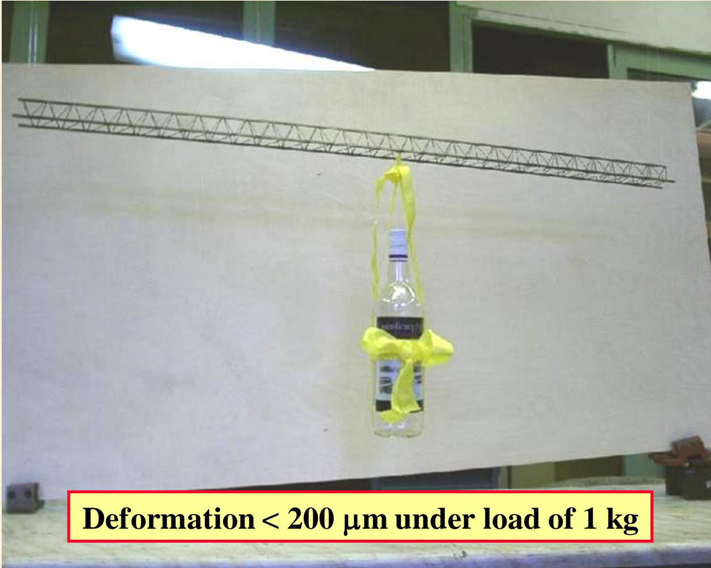
**Deformation  $< 200 \mu\text{m}$  under load of 1 kg**
